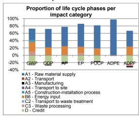
In the production phase, particularly the aluminium components (anodised and in some cases powder-coated with polyester resin) and the material with the highest mass fraction – the MDF board – can be regarded as predominant in terms of their environmental impacts.
